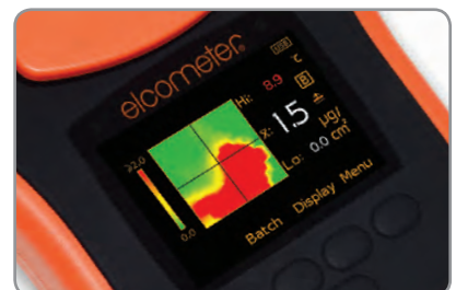
2D Salt Density Map with High/Low Readings
