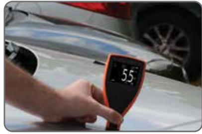
Measures on steel & aluminium body panels 2
