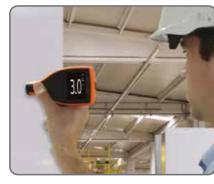
360° auto rotating display for a clear reading at any measurement angle, on the production line or QA station.
