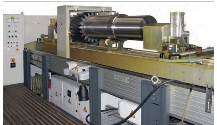
Testing machine with 5000 A for the testing of heavy gear shafts (weight up to 4 t). Customised workpiece holder with special support rolls, which can be changed quickly to ensure highest possible flexibility with respect to the workpiece geometry.
