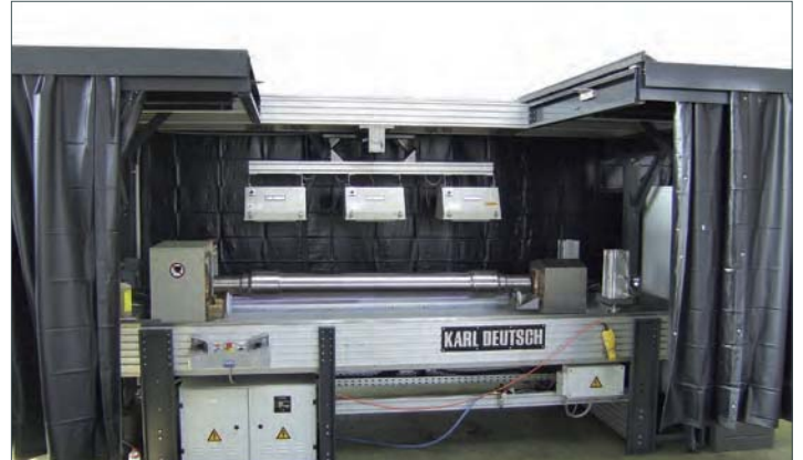
Testing machine for railway axles with motor-driven support rolls. Darkening cabin equipped with pneumatic roof opening and pneumatically movable UV lamps.
