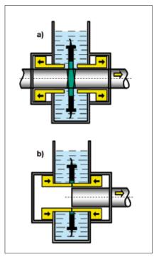
Principle of closing mechanics of test chamber: a) opened test chamber while bar is tested b) bar is leaving the test chamber and one side of chamber is already closed.
