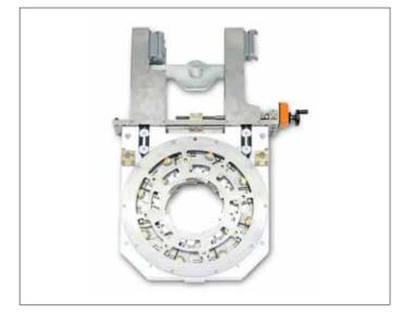
Test cassette with ring of ultrasonic probes. Angle beam probes are used to detect surface defects while straight-beam probes are used to detect core defects. The testing angle of all angle-beam probes is centrally adjusted by the spindle and the orange dial.
