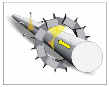
Since the invention of the HRP.S-setup, many probe configurations have been realized. For bar testing, a setup with 16 angle beam probes and 5 straight-beam probes has been proven to be a reliable setup for 100%-cross sectional coverage of the bars. The more probes are used, the higher is the probability of detection (POD) also of oblique and crack-type defects.
