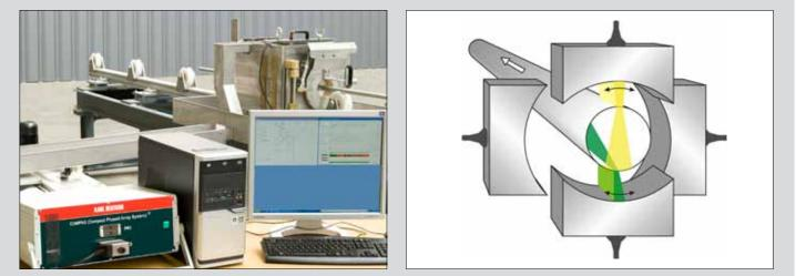
Similar test results can be obtained by using ultrasonic phased arrays. The bar is entirely enclosed by an annular ring array. The phased array technique can then be used to produce straight-beam testing (yellow beam) or angle beam testing (green beam). The advantage of a phased array setup is the fast change-over time for another dimension and to adjust all test parameters electronically. On the other hand, this technique requires many electronic testing channels and extensive probe arrays.
