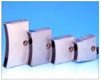
Special line-focussed probes for angular incidence in different sizes to test the respective bar diameters. Each probe covers 30 degree of the bar surface – independent of the bar diameter.
