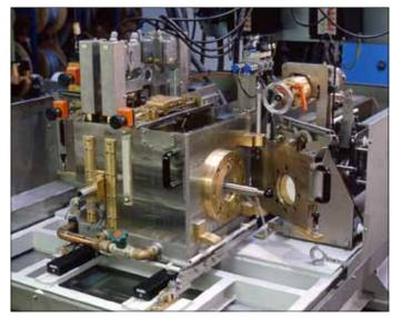
System calibration by means of short bar carrying artificial defects. The bar is rotated such that the defect is passing each ultrasonic probe. Afterwards, the automated sensitivity adjustment equalizes the sensitivity of all probes. For the calibration process, the test chamber is moved into the calibration position (offline).
