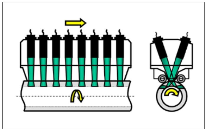
Inspection of tubes for longitudinal defects:
