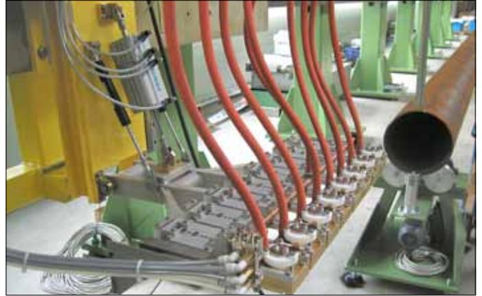
Inspection of tubes with longitudinal weld (ERW tubes):
