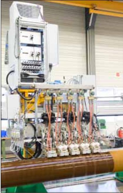
Probe Holders for the detection of longitudinal defects, transverse defects and laminations. Also the wall thickness is measured. In this case, a phased array testing electronics is employed.
