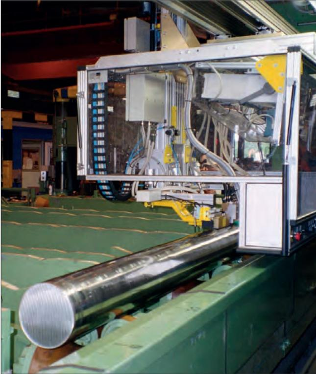
Test portal for steel bars with one common probe holder. The billets are loaded by a transverse conveyor (walking beam) into the test system. After inspection, a linear conveyor discharges the billet.
