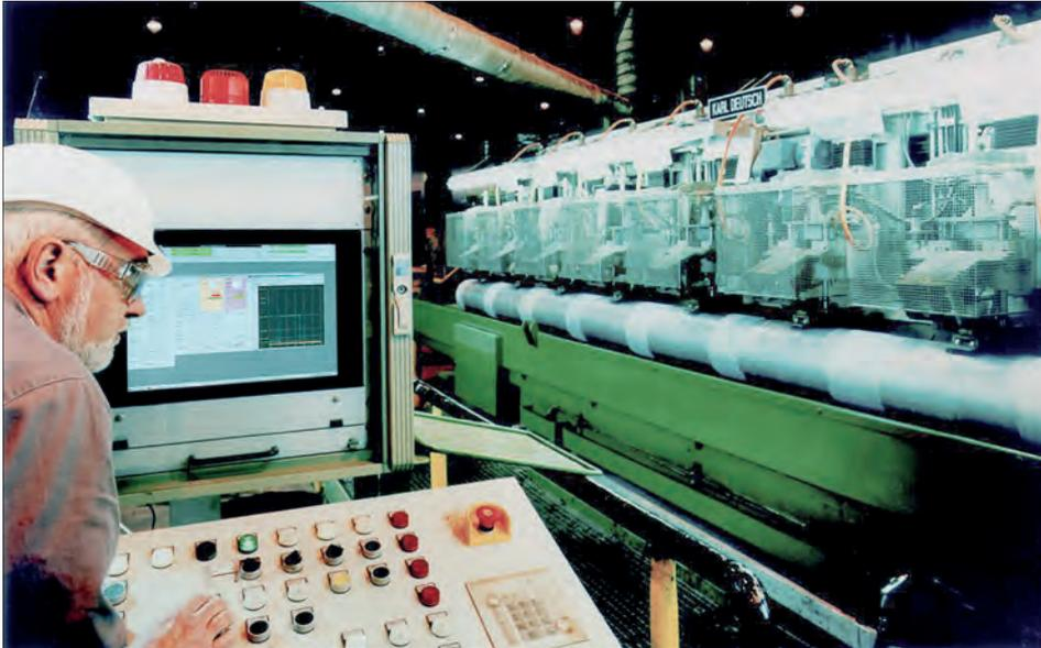
Test portal for round cast aluminium billets with ten straight beam probes for core-defect detection in accordance with ASTM B 594-90. In addition, six angle beam probes inspect the billets for surface defects in critical areas of the billet.
