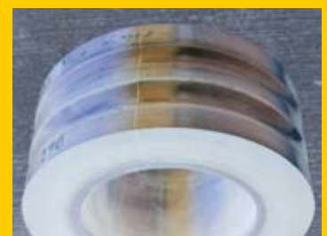
Defective roller with crack
