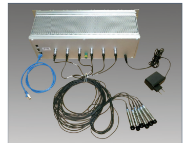
View of the rear of a 19" rack with the connectors for network integration (LAN), control via USB, up to six probes and the power supply (mains plug unit)
