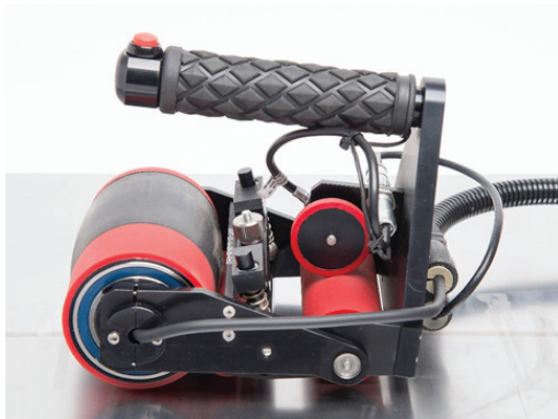
Roller probe for testing on plane surfaces
