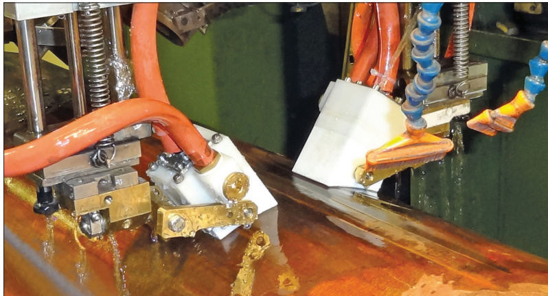
Water Nozzle for probe 1598.666 and 1598.649 with customer specific radius, e.g. for mechanized testing of longitudinal tube welds
