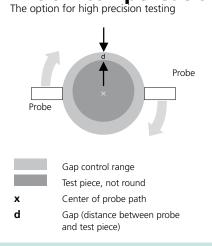
The optional lift-off compensation corrects distorted signals that arise from a varying gap between the probe and test piece. The smaller the gap, the larger the defect signal. If the test pieces are off-center, defects of the same size produce different signal amplitudes, resulting in inaccuracies in the defect evaluation. The lift-off compensation system corrects this effect and ensures reliable test results.
