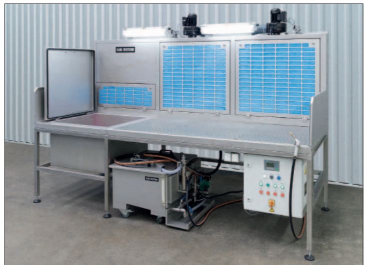
Test station with dip tank for red dye testing and visual evaluation under white light
