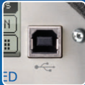
Firmware-updates via USB interface on the rear side
