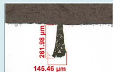
Cross section 2 Defect depth: 0.26 mm
