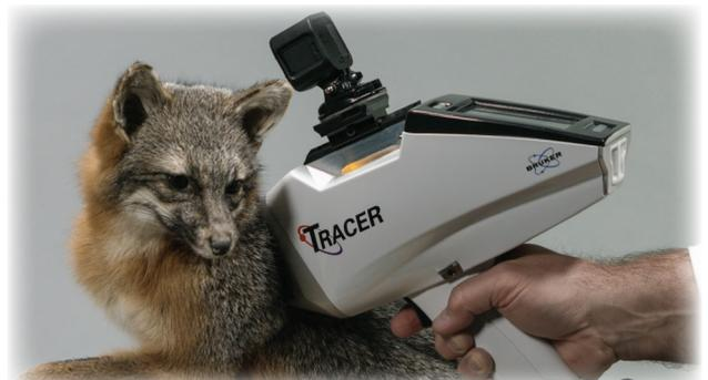
**TRACER 5 checking for poisons on object under NAGPRA program**
