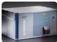
**S2 PICOFOX™** mobile benchtop TXRF analyzer from Bruker with micro focus X-ray tube, multilayer X-ray optics for beam focusing and monochromatization. It simultaneously measures elements from magnesium (Mg) to uranium (U) at ultralow concentrations, as low as parts-per-billion, to high percentage levels. This analyzer is ideal for liquids, suspensions, powders, particles, metals, thin layers, tissues, wipes, filters and more.
