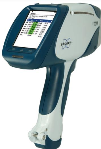
TRACER 5 Handheld XRF analyzer (Na to U)
