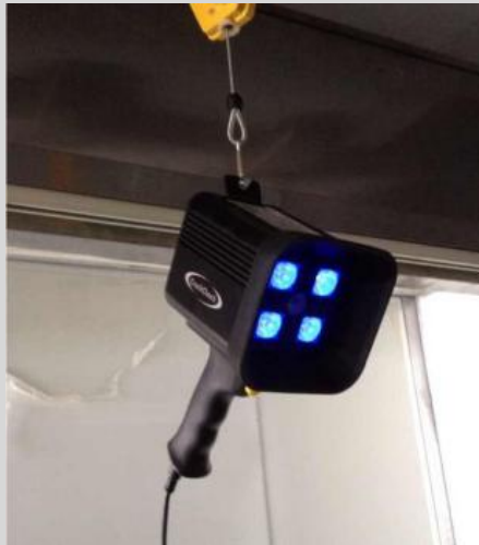
Mounting with spring balance and hook
